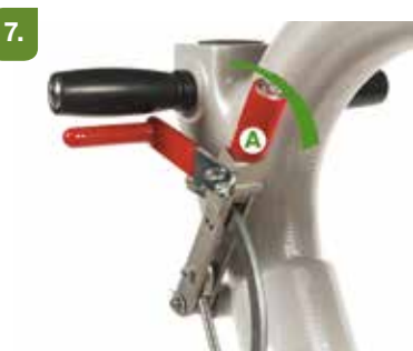
Lift the drum with the lever (A).
