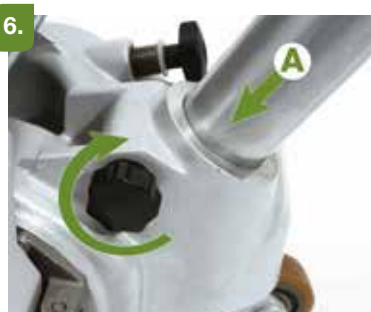
Fit the suction pipe (A) and drum control rod (b).
