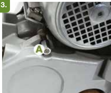
Secure the motor by tightening the knob (A) .
