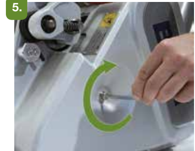
Close the belt guard and tighten the screw.
