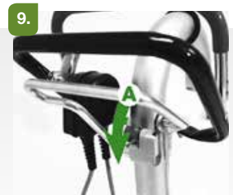
9. Lift the drum with the lever (A).
