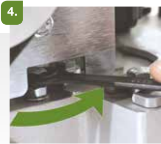
4. Turning the adjustment screw counter-clockwise raises the drum end on the motor fan side from the floor.
