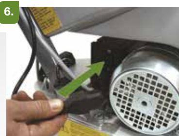
6. Connect the motor plug to the socket on the head of the extractor. Connect the handle/motor interconnection cable to the socket on the side of the motor box.
