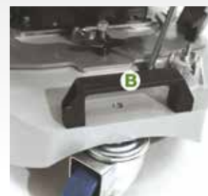
8. Remove the handle from its housing by moving it backwards slightly (A) and then lifting it vertically (B).
