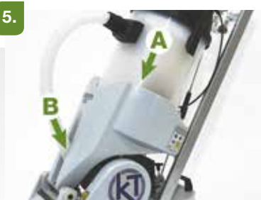
5. Insert the extractor into the basket holder (A), (B).
