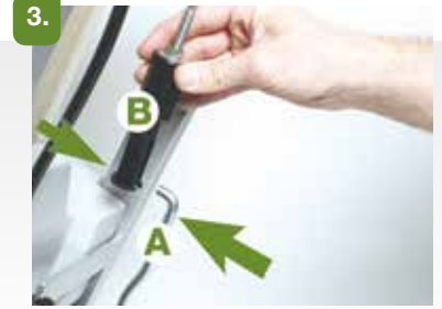
3. Insert the rod (A) into the coupling (B) and lower the tube (C), tightening everything securely.
