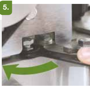
5. Once the desired position has been reached secure the locking nut.
