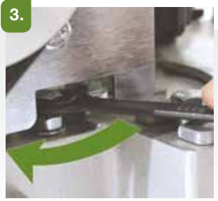
3. Turning the adjustment screw clockwise lowers the drum end on the motor fan side towards the floor.
