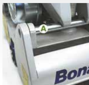
8. Remove the handle from its housing by moving it backwards slightly (A) and then lifting it vertically (B).
