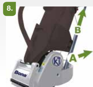
8. Remove the handle from its housing by moving it backwards slightly (A) and then lifting it vertically (B).
