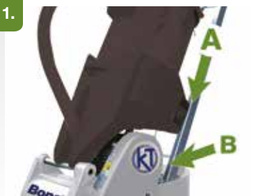
1. Insert the handle into the side guides in sequence (A), (B).
