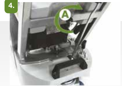
4. Insert the basket holder in its housing on the handle and secure it with the screw knob (A).
