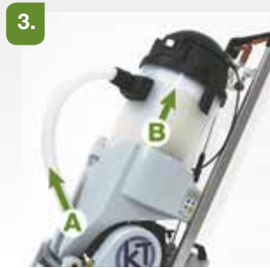
3. Remove the flexible hose from the outlet on the extractor trunk (A) then lift the extractor from its housing (B).
