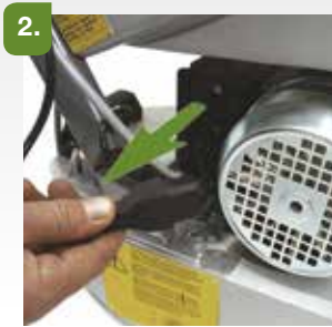
2. Disconnect the motor cable on the head of the extraction unit from the auxiliary socket on the base frame.
