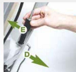
6. After releasing the knob (A) and moving the drum lifting lever forwards (B), lift the tube (C) and release the rod (D) from the coupling (E).
