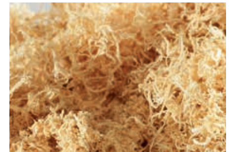
Competitor's sanding dust shows evidence of fibre ripping.
