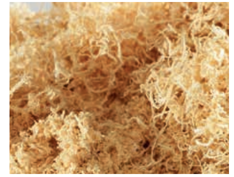
Competitor's sanding dust shows evidence of fibre ripping.
