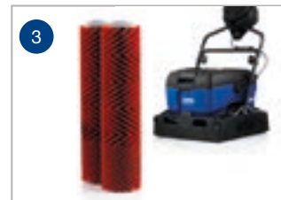
3 Neutralize the floor using Bona PowerScrubber with clear water
